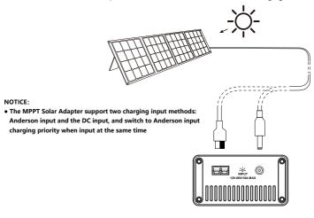
2. Connect the MPPT Solar Adapter and BT01 Battery Pack with Anderson-XT60 charging cable.
