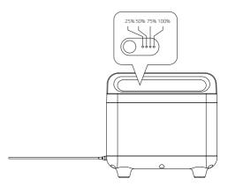
4. When the battery is turned on, the power indicator will always on. Please long press the battery power button 5s to turn off when storing the battery.
